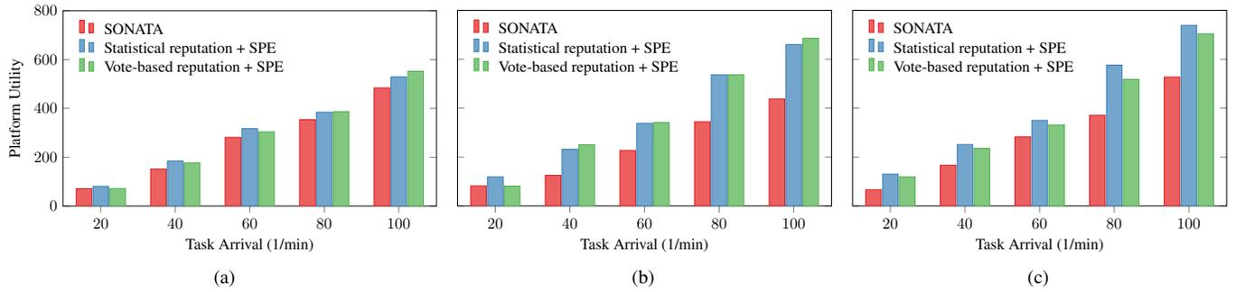
Figure 2. Platform utility vs. sensing task arrival rate for malicious user ratios of a) 3%, b) 5%, and c) 7%.
