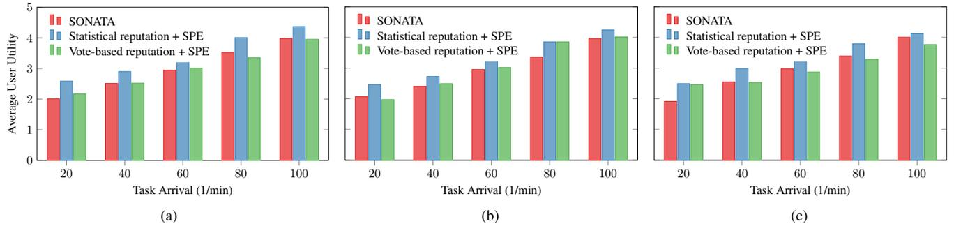
Figure 3. Average user utility vs. sensing task arrival rate for malicious user ratios of a) 3%, b) 5%, and c) 7%.
