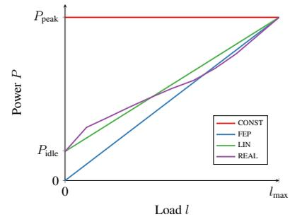
Fig. 1. Power consumption profiles for the IT equipment
